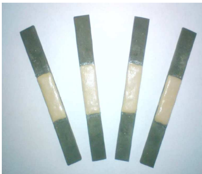
Rysunek 4. Próbki po odlaniu i napaleniu porcelany [5] Figure 4. Samples after casting and porcelain placement [5]
