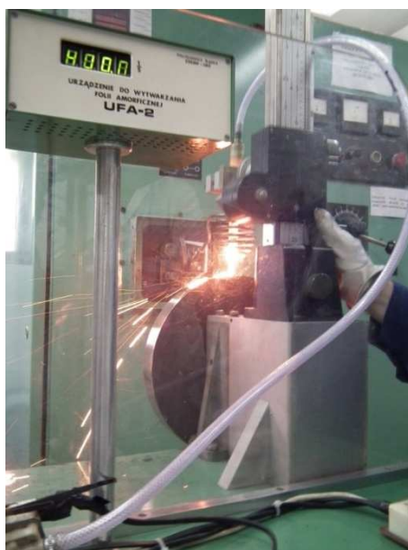
Rysunek 2. Odlewanie taśm ze stopu Co_{68}Fe_4Nb_4Si_{10}B_{14} za pomocą metody melt-spinning Figure 2. Casting of Co_{68}Fe_4Nb_4Si_{10}B_{14} alloy ribbon by the melt-spinning method
