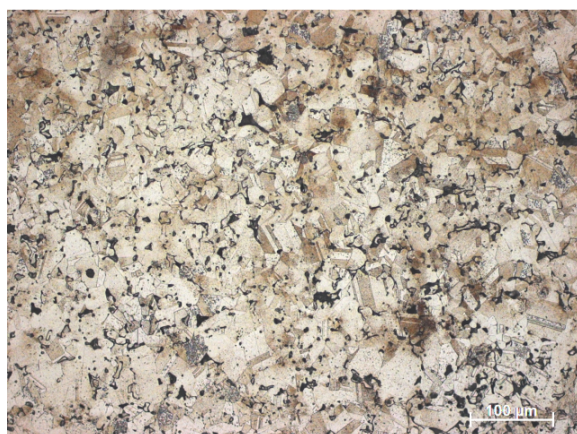
Rysunek 6. Struktura stali X2CrNiMo17-12-2, pow. 100x Figure 6. Microstructure of X2CrNiMo17-12-2 steel, mag. 100x
