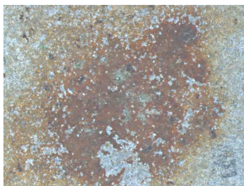
Rysunek 9. Topografia powierzchni po badaniu, stal X6Cr13, pow. 10x Figure 9. Surface topography before testing, of steel X6Cr13, mag. 10x
