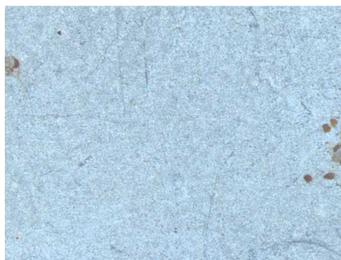
Rysunek 11. Topografia powierzchni po badaniu, stal X2CrNiMo17-12-23, pow. 10x Figure 11. Surface topography before testing, of steel X2CrNiMo17-12-2, mag. 10x
